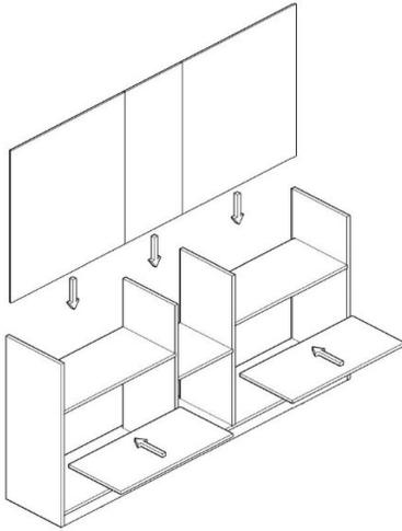
The backboard is inserted into side trays and backboard channels opened on the bottom tray. Shelf pins are attached and moving shelves are placed.
