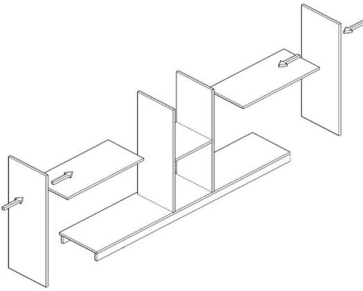
Large baffles and side trays are placed and fixed with the help of a screwdriver.
