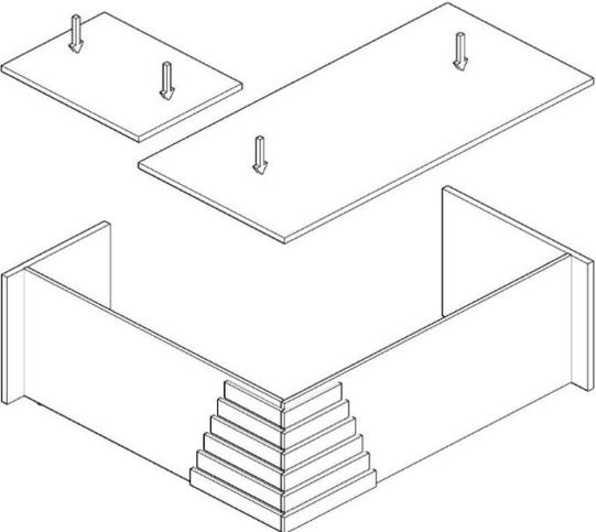
The table top tray and etagere top tray are placed on the connected module and the minifikes are tightened with the help of a screwdriver. The two top trays are connected to each other by using an artek connection plastic and a 6.3 \* 19 ysb screw.
