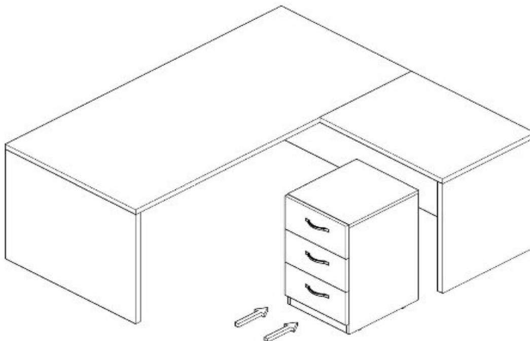
The installed caisson is placed underneath the etagere. Optionally, the caisson drawers can be removed and tightened by inserting 4 \* 35 screws from inner part to the stands and the top.
