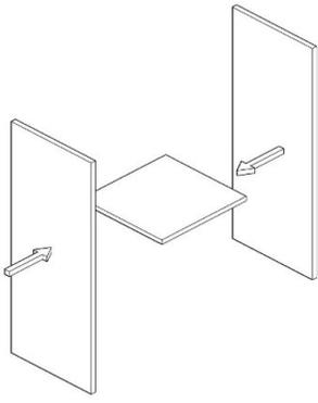
Pillars and short baffle are connected to each other with minifix.
