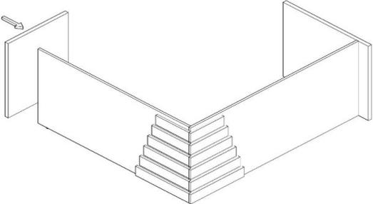
The stand and covers of the product are connected to each other by fixing etagere stand to the module.
