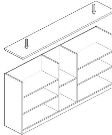
Top tray is placed and are tightened with the help of a screwdriver.
