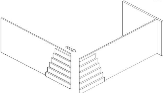
The fixed front cover and the stand are connected with the minifiks.
