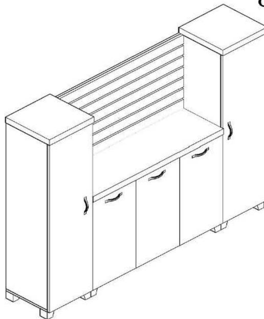
One piece of brake hinge is used on each door. The doors are connected to the side trays and the pillar with 3.5 \* 18 screws. Half camel hinge is used for the single door in the middle and butt hinge is used for all other doors. The handles are fixed to the doors by using 22mm button-head handle screws.
