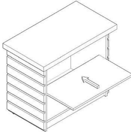
The crystal shelf pins are placed in the holes drilled into the side trays and attached to the moving shelf pins.
