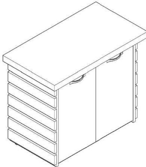
One brake hinge and one butt hinge are inserted on the doors and the doors are connected to the side trays by using 3.5\*18 screws. The handles are fixed on the doors by using 22mm button-head handle screws. They are brought to the miter by adjusting through the hinge.
