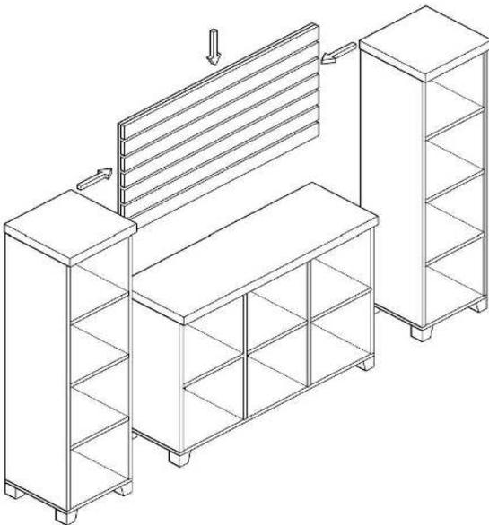
The assembled cabinets are gathered together, and the rear panel and the cabinets are connected with the minifix. 4\*30 screws are used for connecting through inner side of the cabinets.
