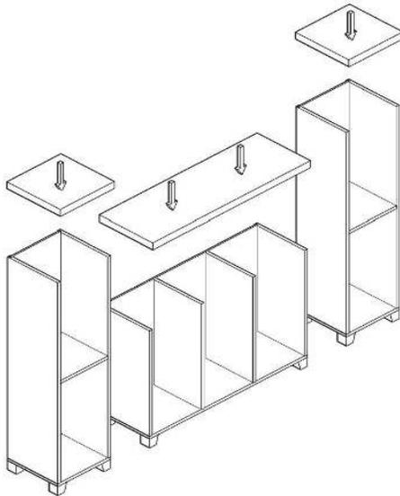
The top tray is placed on the sides and minifixes are tightened with the help of a screw by paying attention to the backboard channel.
