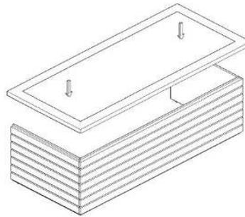
Top tray is placed on the stand and the cover and the minifixes are tightened with the help of a screwdriver.
